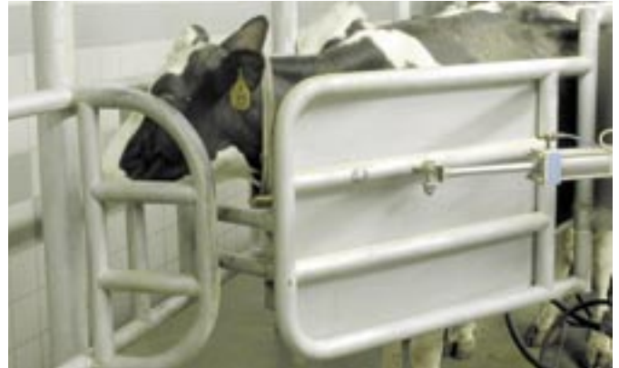
With Conventional Exit, you simply open the exit gate with manual or air-powered gate linkage and the cows exit.
