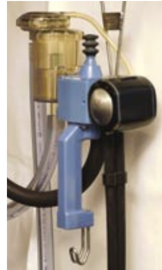
▲ Duovac, first introduced in 1977, automatically adjusted vacuum level to milk flow and was therefore gentler on the cow.
